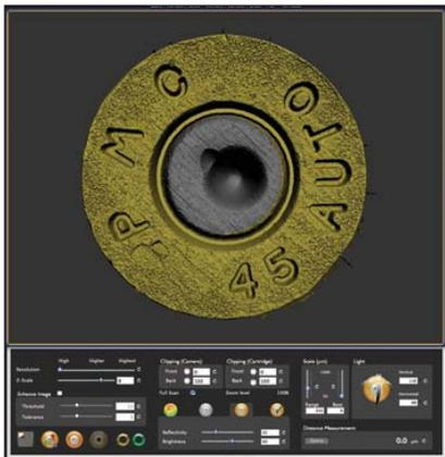
**Forensic ballistic experts** have a new tool to consider. The ALIAS Advanced Ballistics Analysis System from Pyramidal Technologies is a full 3D imaging, correlation, visualization, and confirmation system that builds visually rich expended cartridge and fired-bullet images, then provides powerful software tools to analyze them using topographically sensitive colorization, and adjustable light source and axis orientation.
