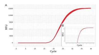
Unparalleled uniformity. Amplification curves for 96 replicates shown on a linear plot (A) and a logarithmic plot (Figure B). In each well, 105 copies of GAPDH template were amplified in the presence of GAPDH primers and BioRad™ Sso Advanced SYBR Green Mix®. Average Cq = 19.1, Coefficient of variance (Cv)= 0.002.
